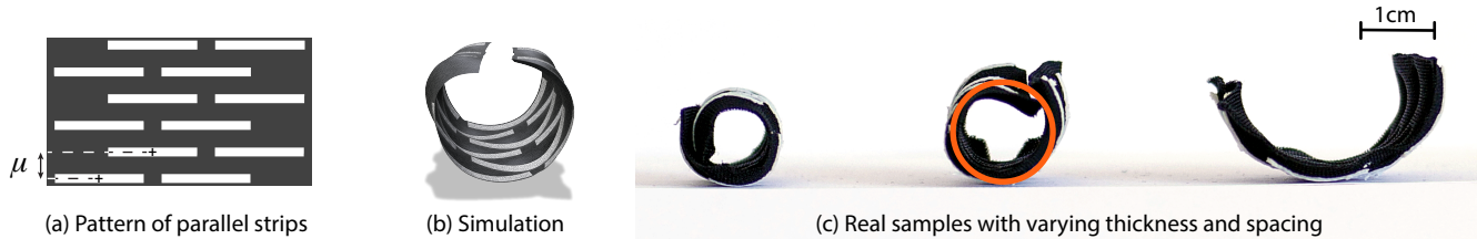
Figure 9: We focused our evaluation on a pattern of parallel plastic strips (a), which rolls as a cylinder when released. Our simulation reproduces well this behavior (b). We fabricated multiple such cylinders by varying the thickness h_p and spacing \mu of the strips (c), and measured their curvature by fitting a circle on their silhouette (c, orange circle).
