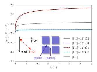
Figure 6: Time evolution of the dislocation densities  $\rho^{\alpha}$  for different directions of the applied load.
