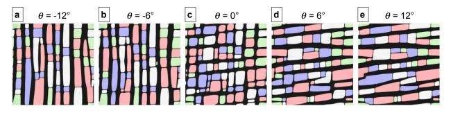
Figure 5: Microstructures obtained at t = 7.6 h with an inhomogenous elastic simulation with no plasticity for several misorientations  $\theta$  of the loading axis a)-12°, b)-6°, c) 0°, d) +6°, e) +12°.
