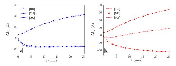
Figure 2: Evolution of  $\Delta L_2(t) = (L_2(t) - L^0)/L^0$  in the three cubic directions for the a - [110] and b - [110]+12° applied load.
