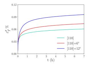
Figure 8:  $\varepsilon_{\vec{\tau}}^P$  along the tensile direction vs time for different applied loads and an initial dislocation density of  $\bar{\rho}_0 = 2.5 \ 10^{12} \ \mathrm{m}^{-2}$ .
