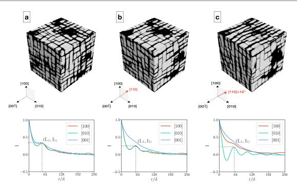
Figure 1: Top: concentration field of a - the initial cuboidal microstructure and the microstructure obtained with the full elasto-viscoplastic model after t = 25.5 min under b - [110] and c - [110]+12° tensile creep loading. Bottom: corresponding autocorrelation functions along the cubic axes.
