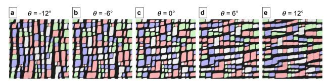
Figure 4: Microstructures obtained at t = 7.6 h with an inhomogenous elasto-viscoplastic simulation for several misorientations  $\theta$  of the loading axis a) -12°, b) -6°, c) 0°, d) +6°, e) +12°.
