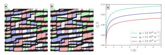
Figure 9: Snapshots of the final microstructure after t = 7.6 h under [110]+12° creep load: a -  $\bar{\rho}_0 = 2 \times 10^{12}$  m<sup>-2</sup> and b -  $3 \times 10^{12}$  m<sup>-2</sup>; c - corresponding evolution of the average plastic strain  $\varepsilon_{\vec{T}}^P$ .
