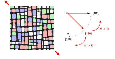
Figure 3: Left: Initial microstructure (colors indicate  $\gamma'$  variants) in 4.6<sup>2</sup>  $\mu$ m<sup>2</sup> periodic box. Red arrows represent the applied stress for the perfect [110] crystal orientation. Right: Diagram of the different misorientations applied to the microstructure.
