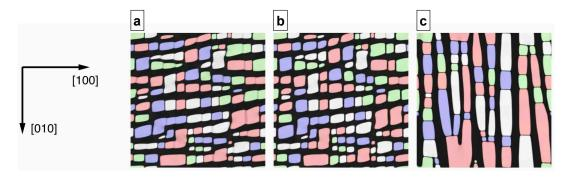
Figure 7: Microstructures in a  $4.6^2 \ \mu m^2$  periodic box after t = 7.6 h under [110]+12° creep load in: a - the homogeneous elasto-viscoplastic case, b - inhomogeneous elasto-viscoplastic case with switched elastic constants; c - inhomogeneous elastic case with switched elastic constants.
