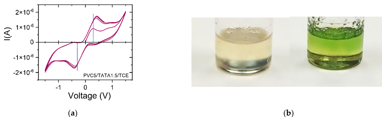
Figure 8. (a) Typical voltammograms obtained at a scanning rate of 100 mV/s, I vs. V , for TATA/solvent and PVC/TATA/solvent samples. The ohmic domain is shown by blue dotted lines. (b) Visual presentation of a freshly prepared gel (left) and the gel after oxidation (right).
