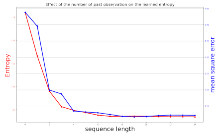
Figure 5: Evolution of the mean differential Shannon entropy associated to the inferred posterior p(X_T|Y_{1:T}) with respect to time horizon T for Lorenz-63 case-study (red). For comparison purposes, we consider the evolution of the mean square error (MSE) of the reconstruction of the true state (blue).
