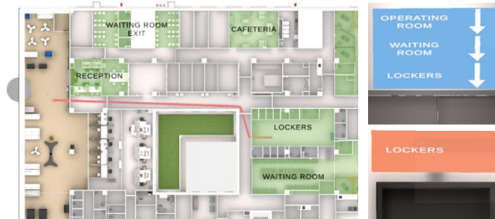
Figure 6. (left) Top view of the model waiting for path selection before generating signs. (right) The blue directional sign and the orange identification sign are generated according to the respective doors.
