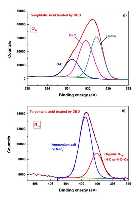
Figure 7: a.  $C_{1s}$  spectrum of terephthalic acid untreated, b.  $C_{1s}$  spectrum of terephthalic acid treated by DBD, c.  $O_{1s}$  spectrum of terephthalic acid untreated, d.  $O_{1s}$  spectrum of terephthalic acid treated by DBD, e.  $N_{1s}$  spectrum of terephthalic acid treated by DBD.
