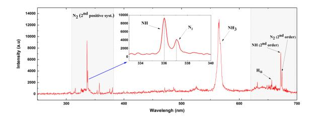
**Figure3.** OES spectrum of terephthalic acid treated by DBD in NH<sub>3</sub>, at 6 kV<sub>pp</sub> voltage, pressure of  $10^4$  Pa, frequency of 4 kHz, and 3 mm of inter-electrode distance.
