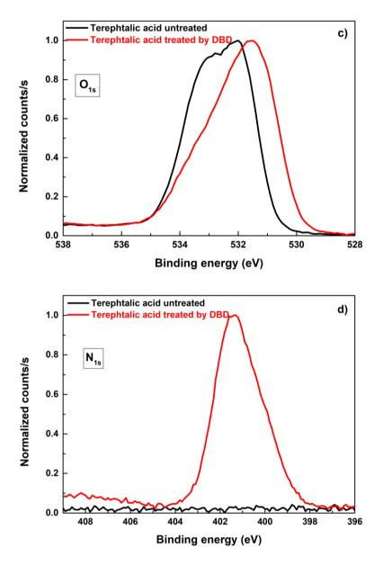
**Figure 6:** a. Survey spectra of terephthalic acid untreated and treated by DBD, b. Normalized  $C_{1s}$  spectra of terephthalic acid untreated and treated by DBD, c. Normalized  $O_{1s}$  spectra of terephthalic acid untreated and treated by DBD, d. Normalized  $N_{1s}$  spectra of terephthalic acid untreated and treated by DBD.
