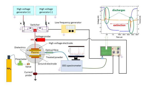
Figure 1. Schematic diagram of the experimental setup of the DBD plasma treatment with electrical and optical diagnostics.
