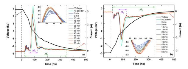
**Figure 2.** Current-Voltage measurements of the DBD plasma treatment of terephthalic acid at  $6 \, kV_{pp}$  voltage, pressure of  $10^4 \, Pa$ , frequency of 4 kHz, and 3 mm of inter-electrode distance. a) falling edge of the voltage, b) rising edge of the voltage. Current measurement without terephthalic acid (green curve) is also shown.
