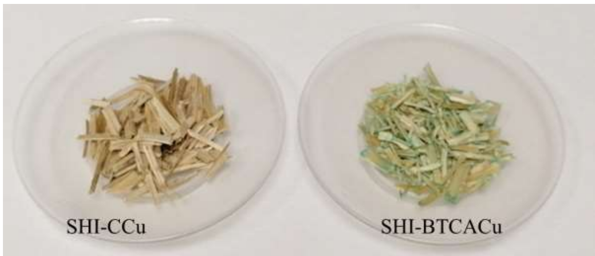
Fig. 2. Hemp shives samples after copper adsorption.
