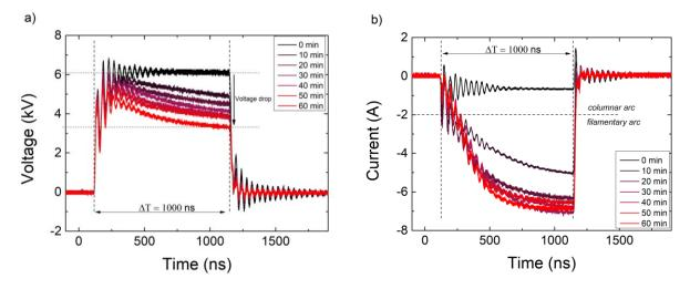
Figure 7: chronogram of (a) the voltage and (b) the current during the plasma treatment of 200 mg of KNG 180 sample in 40 mL of water and in air.
