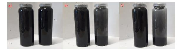
Figure 8: evolution of the graphite dispersion (5 g.L<sup>-1</sup>) in demineralized water after sonication for the treated sample (left bottle) and initial KNG 180 (right bottle), after a) 0 minutes, b) 5 minutes, c) 1 hour.
