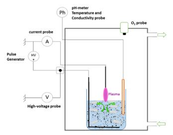
Figure 1: experimental setup for the plasma treatments.
