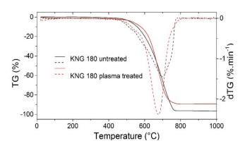
Figure 11: TGA Thermograms (under dry air) of the KNG 180 untreated sample (black) and treated by plasma (red).
