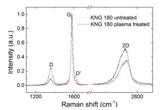
Figure 10: Raman Spectra ( $\lambda$  = 488nm) of the KNG 180 untreated sample (black) and treated by plasma (red).
