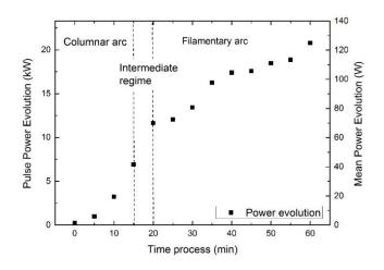
Figure 3: pulse power and the associated mean power evolutions during the plasma treatment process of 25 mg of KNG 180 in 80 mL of water and in air gas.
