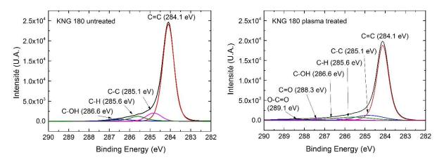
Figure 12: XPS C (1s) decomposed spectrum of the KNG 180 untreated sample and treated by plasma.
