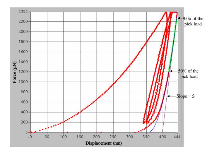
Figure 4. Representation of the typical curve representing the load – displacement performed
