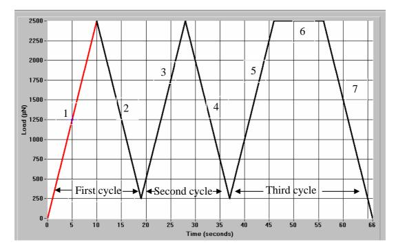
Figure 3. The load cycle applied to the indenter
