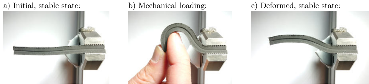
Figure 3. Illustration of the deformation storage in the MagnetoFriction Shape Memory Polymer (MF-SMP).
