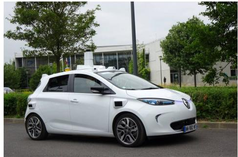
Fig. 8. Autonomous Electric Renault Zoe
