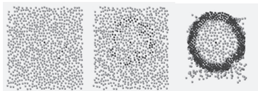
Figure 1: Sequences of direct self-organization of mobile robots into a circle
