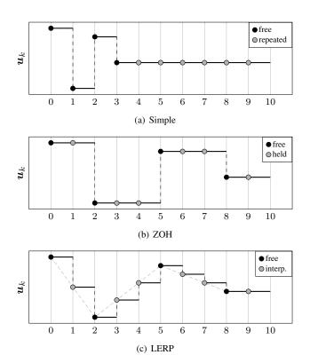
Fig. 1. Example of control sequences  $\underline{u}$  with a reduced number of degrees of freedom. Even if the prediction horizon is  $N_p=10$ , only 4 variables are freely assigned, while the remaining ones are defined in function of the free samples.
