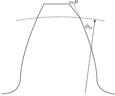
**Figure 3:** Schematic representation of a tip relief modification.  $\mu$  is the amount of tip relief,  $\phi_{tr}$  is starting radius of the profile modification ( $\phi_{tr} = 50.26 \mu\text{m}$ ).
