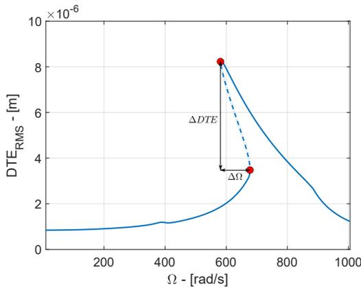
**Figure 4:** Example of forced response curve without tip relief modification ( $\mu = 0 \mu\text{m}$ ). Solid and dashed lines denote stable and unstable responses, respectively. Saddle-node bifurcation points are represented by red circle markers.
