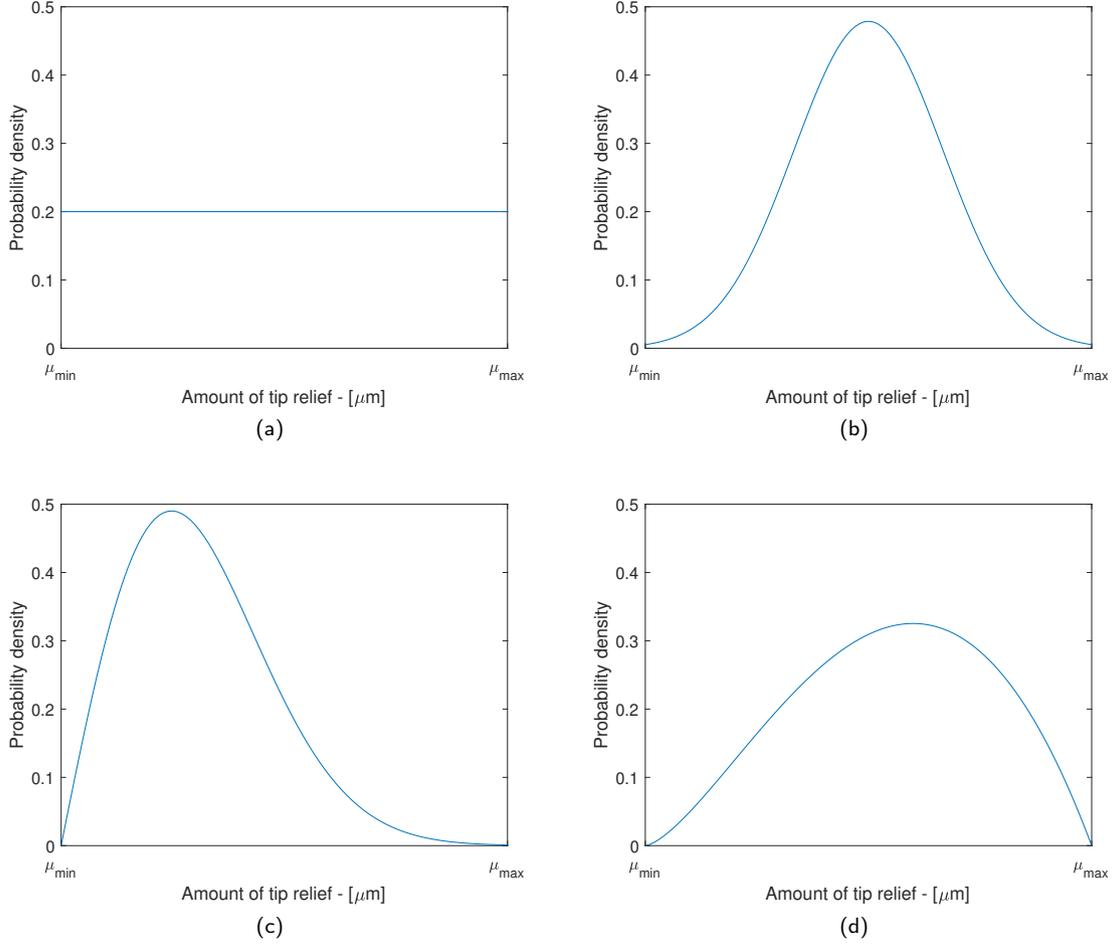
**Figure 5:** Probability density functions considered for the uncertain tip relief parameter. (a) Uniform distribution (b) Normal distribution, (c) Weibull distribution with parameters  $\lambda = 1.75$  and  $k = 2$ , (d) beta distribution with parameters  $\alpha = 2.5$  and  $\beta = 2$ .
