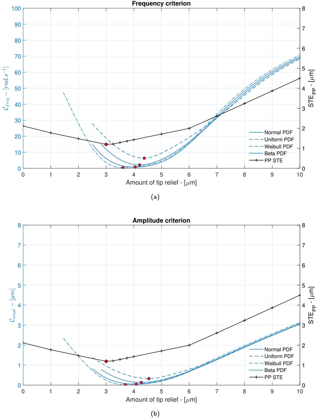
**Figure 8:** Evolution of the frequency criterion (a) and amplitude criterion (b) with respect to the amount of tip relief. Red circle markers denote the optimal value of tip relief. The evolution of the peak-to-peak STE is represented as a black line with cross markers.
