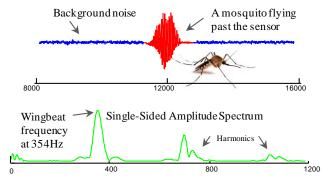
Figure 6: *top*) An audio snippet of an insect flight sound can be converted into a pseudo time series (*bottom*) and used to allow classification
