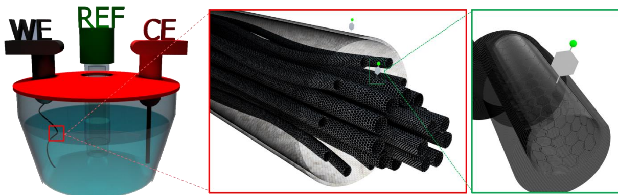
Figure 1. Modified CNTFs with p -substituted phenyl ring through electrochemical reduction of aryl diazonium salt. Green ball corresponds to a general functional group.
