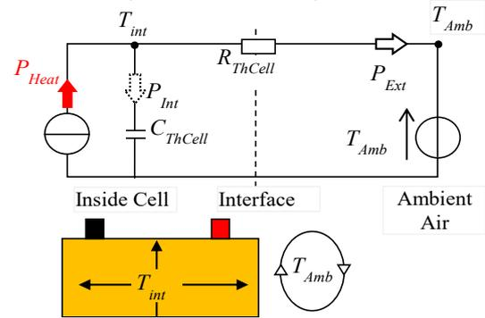
Fig. 2 Structure of the thermal model for one cell [21]
