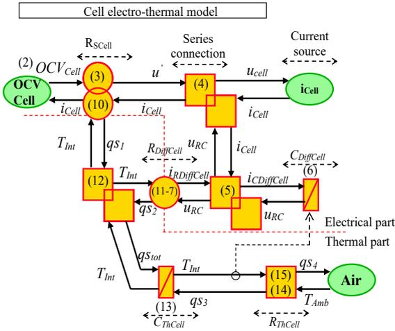
Fig. 5 EMR of the dynamical electro-thermal model [21]
