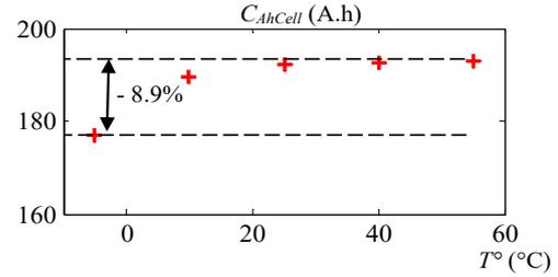
Fig. 9 Evolution of capacity with ambient temperature
