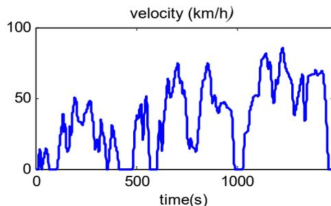
Fig. 18 WLTC driving cycle
