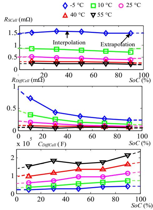
Fig. 12 Impedance parameters with SoC and temperature
