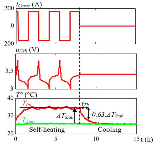
Fig. 13 Thermal characterization protocol
