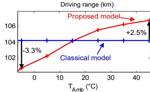
Fig. 20 Driving range as a function of ambient temperature
