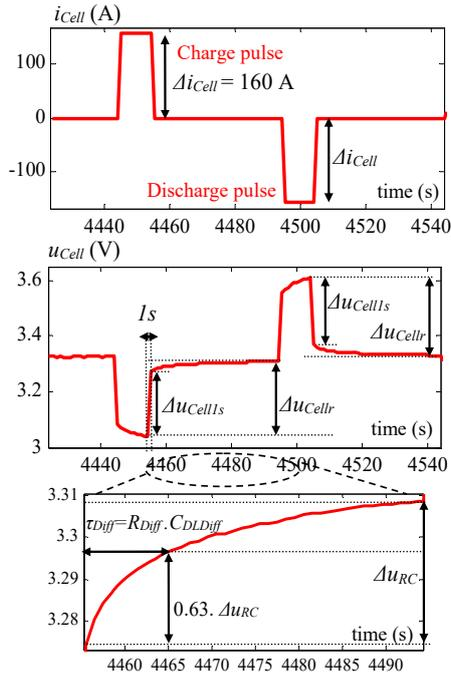
Fig. 11 Characterization pulses
