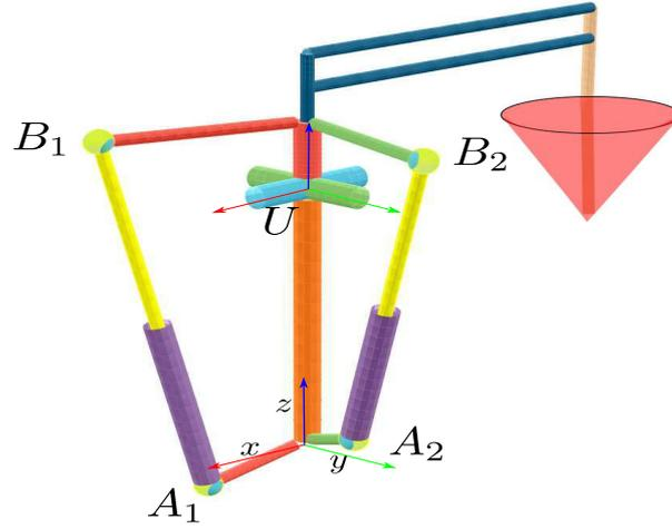
FIGURE 3 – The parameters to be optimized in 2UPS-1U
