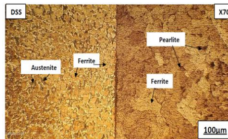
Fig. 3 Microstructures of the dissimilar weld of duplex stainless steel with X70 steel, joined by solid-state diffusion bonding process at 1150^\circ\text{C} for 5 h.
