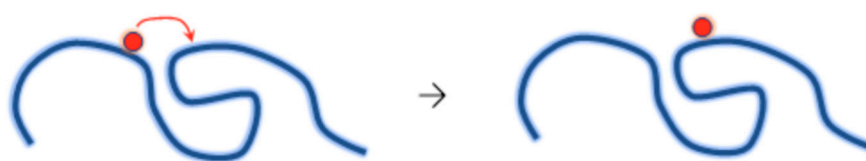
Figure 17. H-transfer leading to a shift in location of the radical along a polymer chain.
