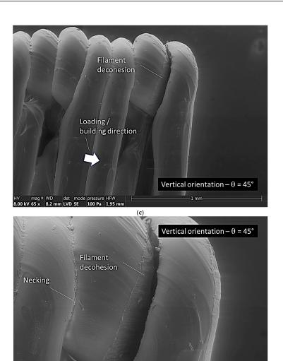
**Figure 5.** Fractured surfaces of samples printed according to the vertical orientation (i.e., building direction parallel to the loading direction): (a) zoom-out; and (b) zoom-in views at the central part of the printed sample; (c) a shifted view at the edge of the sample; and (d) a zoom-in view of the edge highlighting the filament decohesion along the neck.
