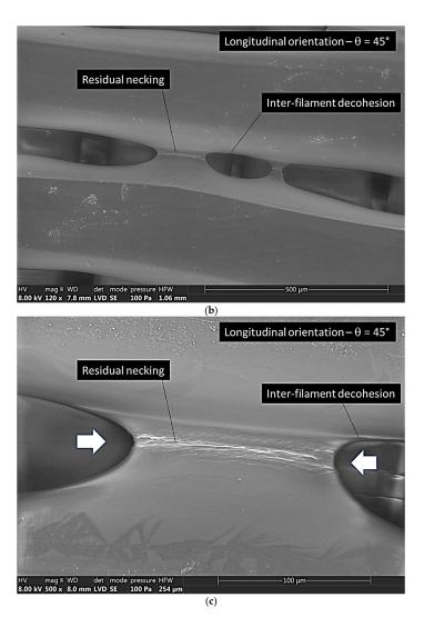
**Figure 8.** Top view normal to the raster showing the layup of  $0^{\circ}/90^{\circ}$  corresponding to a printing angle of  $90^{\circ}$ . (a) The formation of inter-filament cracking, which propagates in the loading direction; (b) a magnified view showing the bridging process between longitudinal cracks generated by the inter-filament decohesion; and (c) a magnified view showing the residual necking (region highlighted by arrows) in sandwich between two longitudinal cracks.
