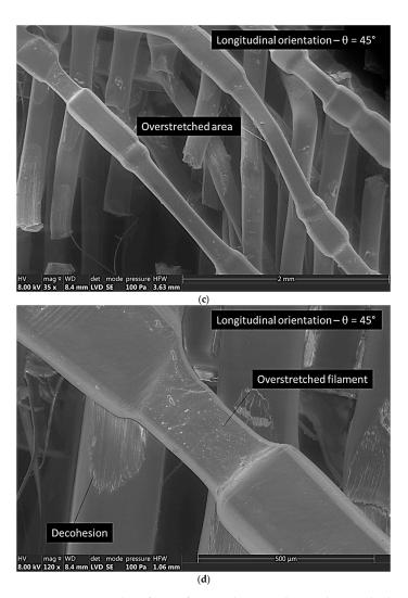
**Figure 7.** Fractured surfaces of a sample printed according to the longitudinal orientation: (a) zoomout at the rupture area; (b) a close view at the ruptured area; (c) a global view of the overstretched filaments; and (d) a zoom-in view on a ruptured filament.
