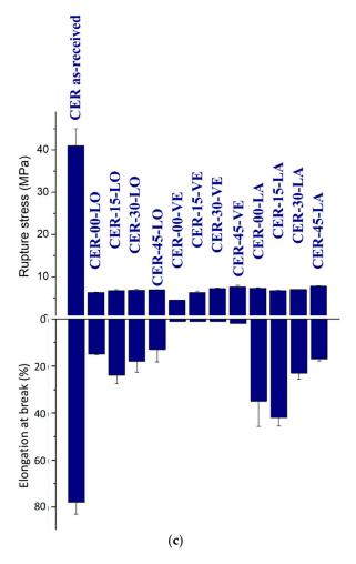
**Figure 11.** Observed tensile performance of CER versus printing conditions. In the nomenclature CER-XX-YY, CER is PLA-ceramic filament, XX is the printing angle, and YY is the printing orientation. (a) The density and Young's modulus; (b) yield stress and tensile strength; and (c) ultimate stress and elongation at break.
