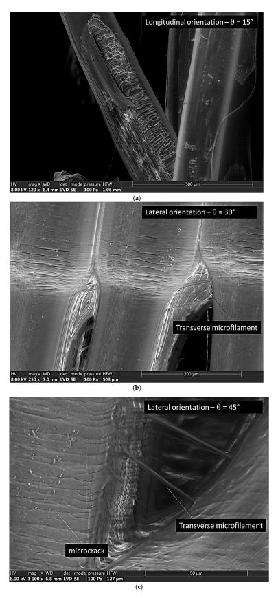
**Figure 9.** Effect of the printing angle on the deformation mechanisms: (a) longitudinal orientation—printing angle of  $15^{\circ}$ ; (b) lateral orientation—printing angle of  $30^{\circ}$ ; and (c) lateral orientation—printing angle of  $45^{\circ}$ .
