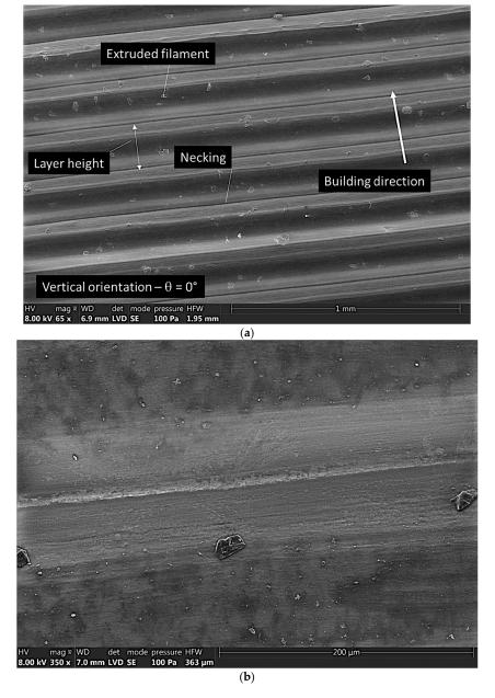
**Figure 3.** Out-of-plane microstructural arrangement showing (a) the filament alignment along the building direction for a sample printed according to the vertical orientation and (b) a close view of the necking structure.
