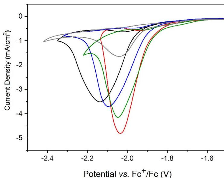
**Figure 3.** Cyclic voltammograms on GC electrode of 1 mM complex [1] and 0.5 M of different supporting electrolytes in acetonitrile solution containing 5 % v/v H<sub>2</sub>O under CO<sub>2</sub>. [TBA][PF<sub>6</sub>] (black plot), [BMPyrr][PF<sub>6</sub>] (gray plot), [EMIM][PF<sub>6</sub>] (red plot), [BMIM][PF<sub>6</sub>] (blue plot) [EMIM][BF<sub>4</sub>] (green plot). Scan rate 0.01 V s<sup>-1</sup>.
