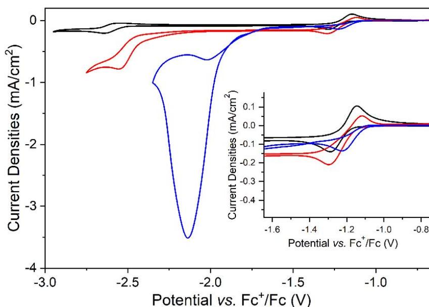
**Figure 2.** Cyclic voltammograms on GC electrode of 1 mM complex [1] and 0.5 M  $[\text{TBA}][\text{PF}_6]$  in acetonitrile under Argon (black plot), under  $\text{CO}_2$  (red plot) and under  $\text{CO}_2$  in the presence of 5% v/v  $\text{H}_2\text{O}$  (blue plot). Inset showing enlarged area on the Rh-centered redox peak. Scan rate  $0.01 \text{ V s}^{-1}$ .
