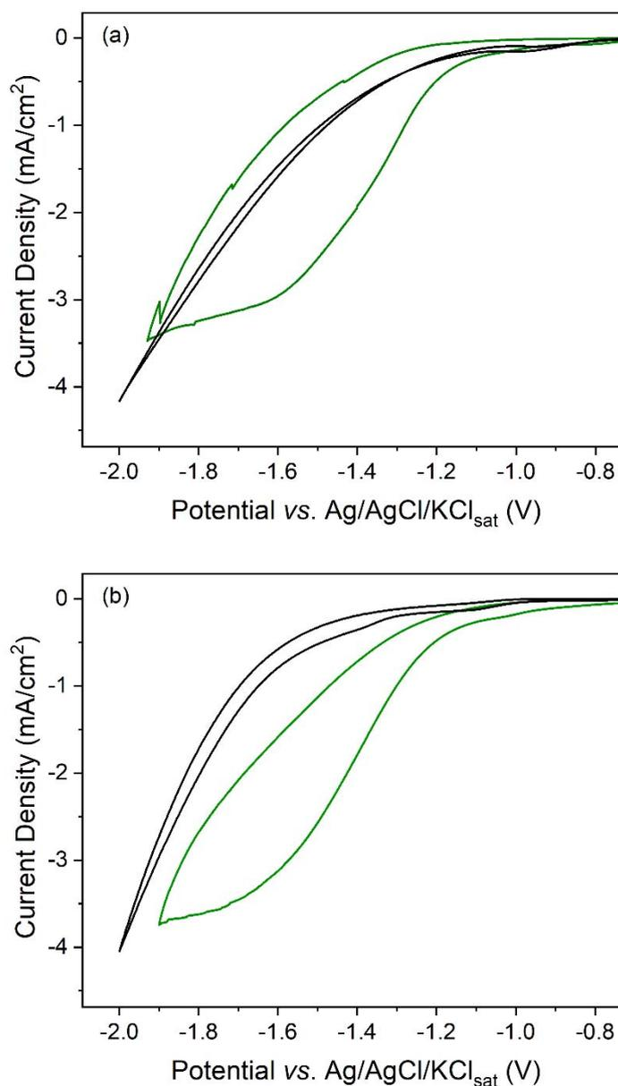
**Figure 4.** Cyclic voltammograms on GC electrode in an aqueous solution containing: (a) 0.1 M [TBA][BF<sub>4</sub>], 0.1 M acetate buffer (pH = 3.8) and 1 mM complex [1] either under Argon (black plot) or under CO<sub>2</sub> (green plot); (b) 0.1 M [EMIM][BF<sub>4</sub>], 0.1 M acetate buffer (pH = 3.8) and 1 mM complex [1] either under Argon (black plot) or under CO<sub>2</sub> (green plot). Scan rate = 0.01 V s<sup>-1</sup>.
