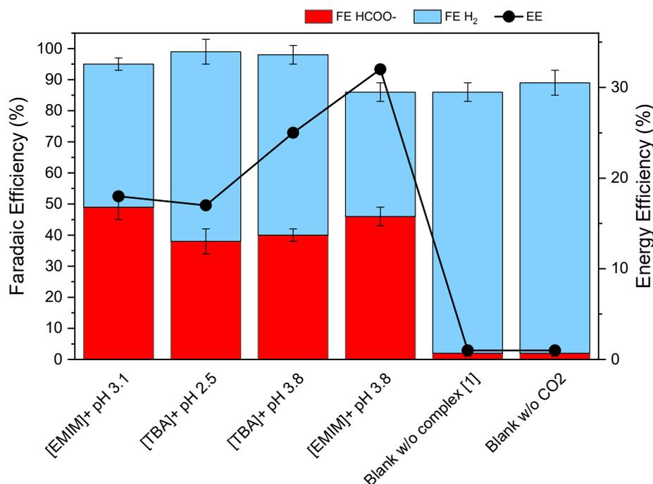
**Figure 5.** FE (%) and EE (%) electrolysis results obtained at  $-3.33 \text{ mA cm}^{-2}$  in  $\text{CO}_2$ -saturated acidic aqueous solution using different electrolytes and proton source in an electrochemical two compartments H type cell.
