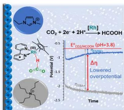
The presence of imidazolium-based ionic liquids in solution significantly impacts on molecular electrocatalysis selectivity and activity by favoring CO<sub>2</sub>RR vs. HER performance in both acetonitrile and aqueous solution. The combination as electrolytes of [EMIM][BF<sub>4</sub>] and acetic acid amplifies their individual roles by enhancing CO<sub>2</sub> conversion to formate at very low overpotential (0.28 V) in acidic aqueous solution.
