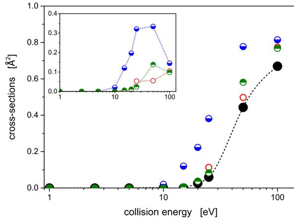
**Figure 6.** Comparison of type 1 momentum-transfer cross-sections and dissociation cross-sections as obtained for  $N_2^+(j=0,v=0)/He$  collisions via the MCSCF/avqz(spdf) method (full and open circles, respectively) and using artificial neural network (ANN) representations of the  $N_2^+/He$  potential energy surface (pluses and crosses, respectively). In the inset, deviations between the ANN and MCSCF/avqz(spdf) data ( $ANN-MCSCF$ ) are depicted.
