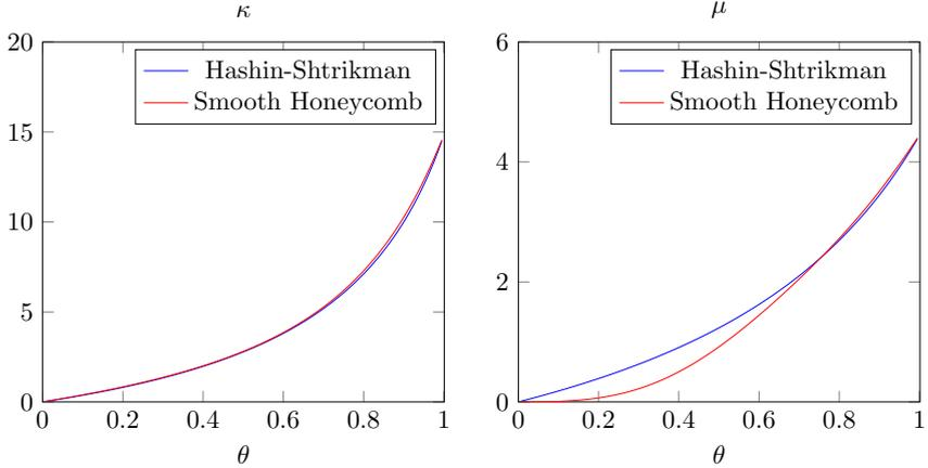
**Fig. 3** The bulk  $\kappa^*$  (left) and shear  $\mu^*$  (right) moduli of the smooth honeycomb wrt. Hashin-Shtrikman bounds
