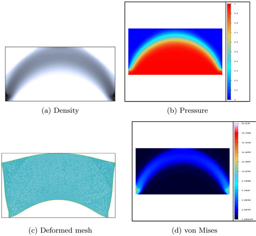
**Fig. 8** (a) The optimal density, (b) pressure field, (c) deformed mesh, and (d) von Mises stress for test case 7.1
