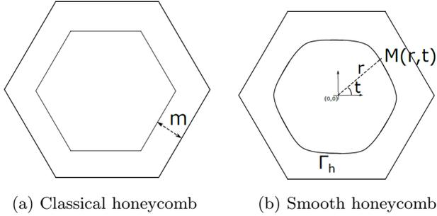
**Fig. 1** Isotropic design cells (images taken from [28])
