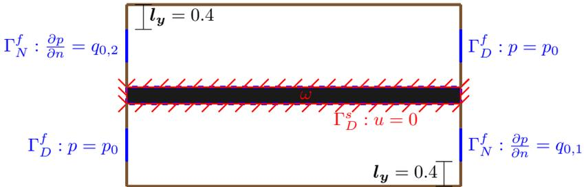
**Fig. 15** Setting of the 2-d counter-flow exchanger 7.4. The brown layers at the walls stand for zero Neumann boundary conditions for the pressure (i.e.,  $\frac{\partial p}{\partial n} = 0$ ); homogeneous Dirichlet boundary conditions hold on  $\partial\omega$ .
