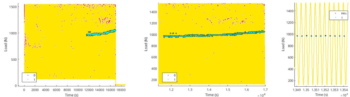
FIGURE 5 – Acoustic activity during a uniaxial tension-tension stress-controlled fatigue test on 5083 aluminum at 0.5 Hz : load vs time. Red dots correspond to all signals recorded above the detection threshold by sensor 1, and blue dots correspond to the signals belonging to the multiplet M1. From left to right : the entire test, and two successive zooms on multiplet M1.
