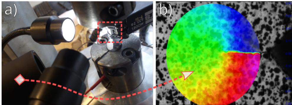
FIGURE 3 – a) Photo of the fatigue test setup with camera and lighting ;
