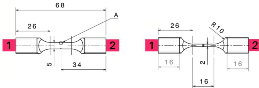
FIGURE 2 – DENT geometry and location of sensors 1 and 2
