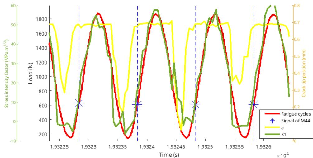
FIGURE 9 – Evolution of the crack tip position  $a$ , the stress intensity factor  $K_I$  and the applied load during a uniaxial tension-tension strain-controlled fatigue test on 42CD4 steel at 1 Hz. The occurrence of AE signals belonging to multiplet M14 are shown as blue stars.
