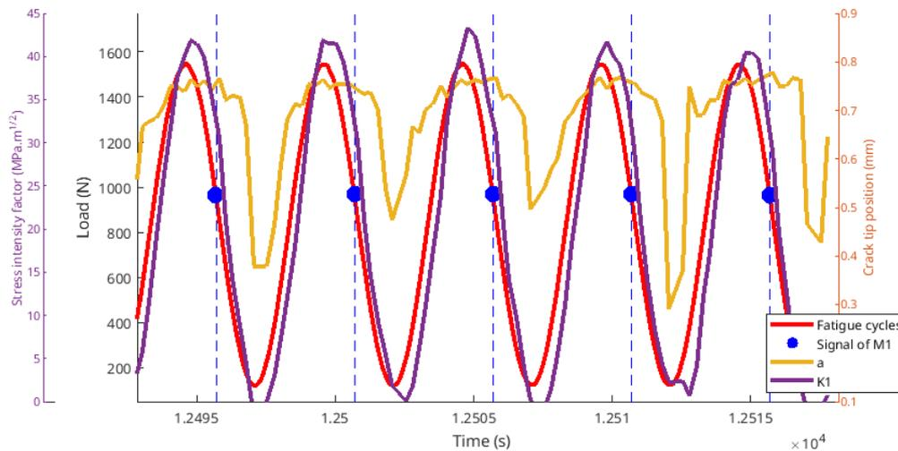
FIGURE 10 – Evolution of the crack tip position  $a$ , the stress intensity factor  $K_I$  and the applied load during a uniaxial tension-tension stress-controlled fatigue test on 5083 Aluminum at 0.5 Hz. The occurrence of AE signals belonging to multiplet M1 are shown as blue dots.
