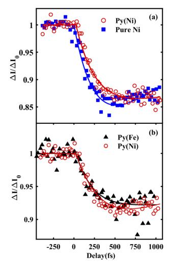
**Fig. 10.** (a) Element-specific demagnetization dynamics of Ni in pure Ni (blue square) compared to Ni in Py (Ni $_{80}$ Fe $_{20}$ ) measured using the resonant Faraday effect. (b) Element-specific demagnetization dynamics of Ni in Py compared to Fe in Py obtained for a similar degree of demagnetization.
