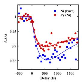
**Fig. 5.** Normalized asymmetry as a function of the time delay for Py (red, circle) and Ni (blue, square) samples measured at the  $M_{2,3}$  absorption edges of Ni (hv = 66.7 eV).
