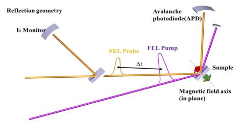
**Fig. 3.** Schematic description of the split and delay experimental setup in the reflection geometry showing the incidence angle on the sample  $(45^{\circ})$ , the  $I_0$  monitor, the direction of magnetization of the sample and the APD recording the reflected signal.
