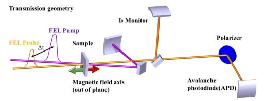
**Fig. 6.** Schematic diagram of the transmission setup showing, in addition to the split and delay unit, the out of plane magnetization of the sample (red and blue), the intensity monitors for pump and for probe, the polarizer (wide band multilayer) and the signal detector (APD).
