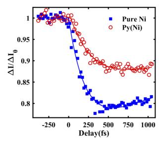
**Fig. 11.** The comparison between Py ( $Ni_{80}Fe_{20}$ ) (red circle) and pure Ni (blue square) measured by Faraday effect with the same pump fluence range (from 1 to 1.5 in units of Fig. 9 (a) and (c)).
