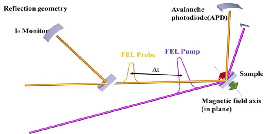
**Fig. 3.** Schematic description of the split and delay experimental setup in the reflection geometry showing the incidence angle on the sample ( $45^\circ$ ), the  $I_0$  monitor, the direction of magnetization of the sample and the APD recording the reflected signal.
