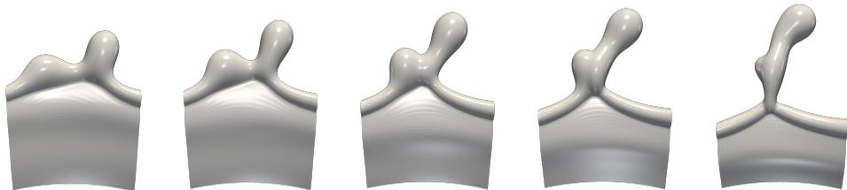
Figure 9: Spatio-temporal evolution of two adjacent rim protrusions which shift in the spanwise direction induced by local cusps, resulting in their collision;  $\theta$  denotes the angle made by the right crest with the rim. The time difference between snapshots is  $\Delta t = 1.0$ . The parameters remain unchanged from figure 2.
