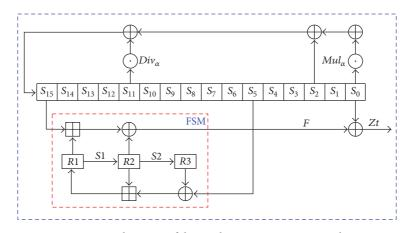
FIGURE 1: Architecture of the regular SNOW-3G stream cipher.
