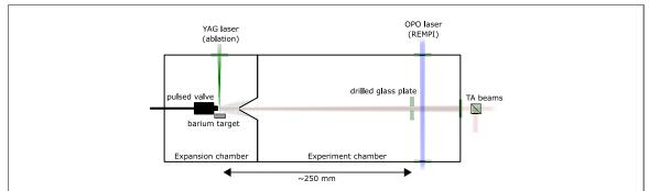
**Figure 1.** Schematics of the experimental set-up. A supersonic beam of BaF is irradiated by up to two light TA beams for vibrational and rotational pumping (see main text and figure 3 for details). The REMPI detection is achieved by an OPO laser and multichannel plates (not depicted).
