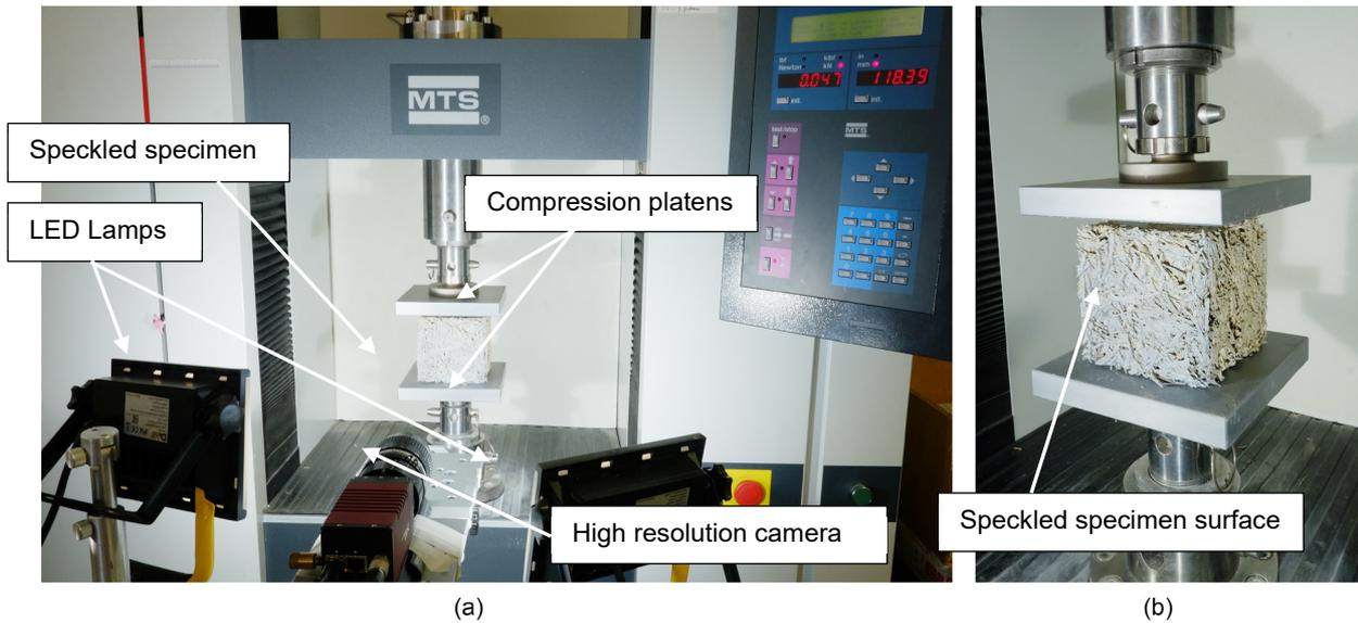
Fig. 2: (a) Set up of specimen compression test and DIC equipment, and (b) black and white speckled specimen
