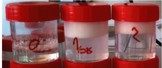
FIG. 2. Typical 10 hours-old samples of dispersions of air micro-bubbles encapsulated with a silicate shell. Those samples were obtained by mixing equal volumes (25 mL) of dispersed HTAC stabilized micro-bubbles with a disodium metasilicate solution (pH adjusted to trigger the silicic acid polymerization). We show the impact of the concentration of disodium silicate, at 0.18 M (#1bis) and 0.09 M (#2). Without any encapsulating protective shells (sample (#0)), the micro-bubbles dispersions disappears in less than 2 hours.
