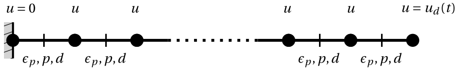
Figure 6. A one-dimensional bar discretized with equal-sized finite elements. Displacements are stored at the node, whereas internal variables are stored at the element integration point (depicted with a vertical bar).
