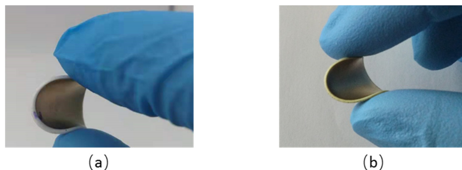
Figure 7. Elaborated flexible samples with 8% vol. of structured composite: (a) ZnO MRs/PDMS and (b) ZnO MPs/PDMS.
