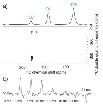
**Figure 6.** (a) Two-dimensional DNP enhanced  $^{13}\text{C}$  refocused INADEQUATE spectrum of Mat(1)-NHC-Ir. Experimental details are given in the legend of Figure S28. The asterisk indicates a spinning sideband. The 1D carbon-13 CPMAS spectrum is shown above the 2D plot. (b) Modulation of the C6" signal intensity recorded in 1D INADEQUATE spectra as a function of the second delay  $\tau_2$ . The first delay  $\tau_1$  was set to 8 ms.
