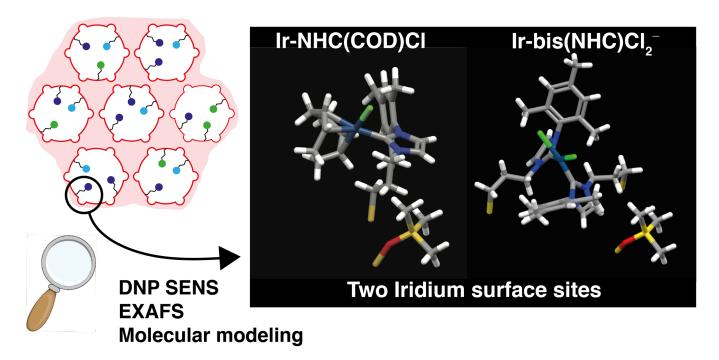
DNP Surface Enhanced NMR Spectroscopy jointly with EXAFS and molecular modeling allows the site-selective structure description with atomic-level resolution of catalytically active iridium supported complexes in a multi-species environment.
