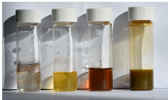
Figure S6. From left to right, colloidal suspensions with C_{\text{full}} = 1 mg/L (without polymer), 25 mg/L (M2, C_{\text{pol}}=0.35 g/L), 0.26 g/L (M4, C_{\text{pol}}=20 g/L) and 1.6 g/L (M5, C_{\text{pol}}=10 g/L).
