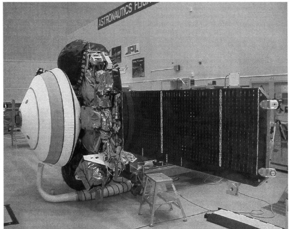
Fig. 1. The Genesis spacecraft is positioned on its side during assembly at Lockheed Martin Astronautics. The white return capsule houses all of the solar-wind collectors. The Genesis electron monitor (GEM) is the exposed instrument at the upper corner of the spacecraft deck. Original color image appears at the back of this volume.
