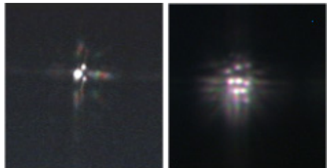
Fig. 4. Laboratory simulated triple (left) and quintuple (right) stars observed with the hypertelescope. The image is a color composite of three images taken through R, G and B filters.
