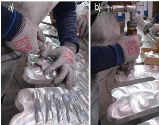
**Fig. 6** Grinding steps by industrial means, **a** vibrating grinder and **b** straight grinder with a grit 40 and grit 80 sandpaper respectively**Table 2** TSA surface treatment sequence of the AA7050-T7451 alloy
