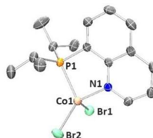
**Figure 2.** ORTEP representation of complex [**L**CoBr<sub>2</sub>] (CCDC 2149630) with 50% ellipsoid probability. Hydrogen atoms are omitted for clarity. Selected bond lengths (Å) and angles (°): Co1-Br1 2.3813(6), Co1-Br2 2.3499(6), Co1-N1 2.036(2), Co1-P1 2.3489(9); N1-Co1-Br2 111.63(7), N1-Co1-P1 85.72(7), N1-Co1-Br1 108.21(7), Br2-Co1-Br1 115.71(2), Br2-Co1-P1 114.30(3), Br1-Co1-P1 117.05(3).
