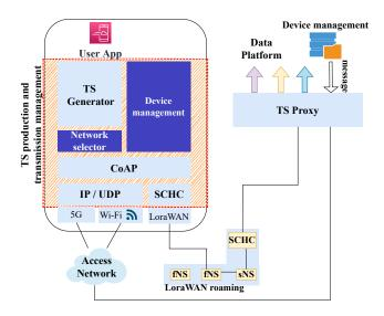
Fig. 1. The proposed IoT architecture.
