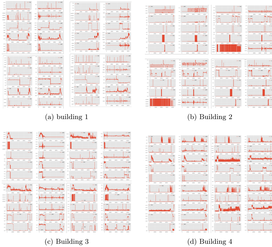
Fig. 5: Selected results on top five appliances of first 4 building of REDD dataset. For each building the appliances are presented in the same order as in table 2. The left panels correspond to the disaggregated target signals and the right panels presents the predicted output from Conv-NILM-net.
