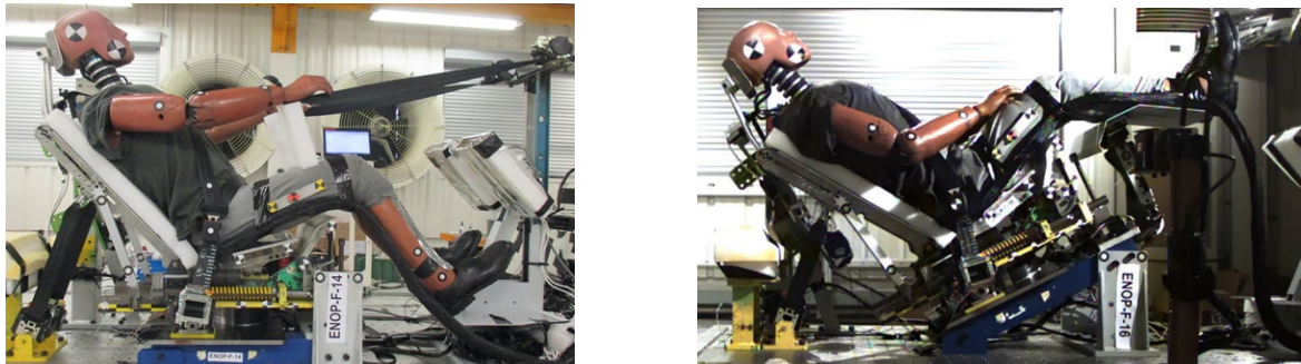
Fig. 2. Left: sled test with HIII-50M positioned in SP2. Right: sled test with HIII-50M positioned in SP5.
