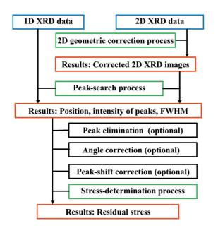
Figure 1 Flowchart of the *X-Light* software. Blue, black, green and red frames, respectively, present the input XRD data, the user-defined parameters, the process algorithm and the results of each process.
