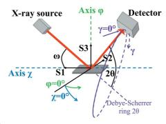
Figure 2 Presentation of diffraction angles at  $\varphi = 0^{\circ}$ ,  $\chi = 0^{\circ}$ .  $\varphi$  and  $\chi$  represent the goniometer rotation.
