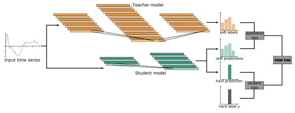
Fig. 1: Overview of our knowledge distillation architecture for time series classification
