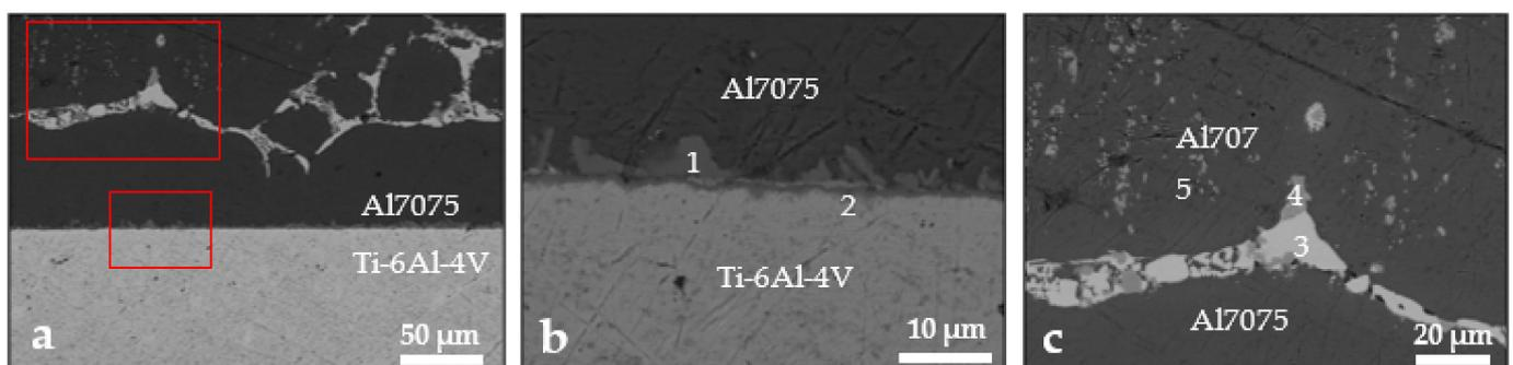
**Figure 3.** Microstructure of the Al7075/Ti-6Al-4V interface with Cu interlayer at 520 °C, holding pressure of 10 MPa, and holding time of 10 min at (a) low magnification at the joint region, at higher magnification (b) at the joint region, and at (c) diffused copper in the Al side. The magnified areas in (b,c) are shown as red rectangles in (a).
