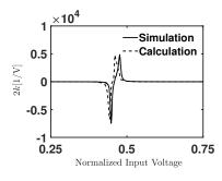
Fig. 5.  $A'_V$ , the second derivative of the voltage transfer characteristic curve with respect to the input voltage.  $A'_V$  is equal to 2k, where k is the scaling factor.
