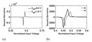
Fig. 2. (a) The second derivative as a function of the normalized  $V_{IN}$  and  $V_{DD}$ . (b) The second derivative of the voltage transfer function as a function of process corners and the normalized input voltage for  $V_{DD}$  of 0.5 V.
