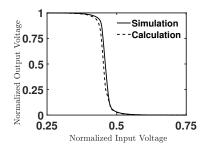
Fig. 3. Simulated and calculated VTC of an inverter cell. The input and output voltage are normalized to  $V_{DD}$  of 0.5 V.
