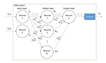
Fig. 3. A system scheme of SNN.
