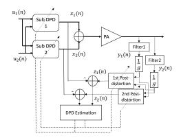
Fig. 1. System of PA and 2D DPD.
