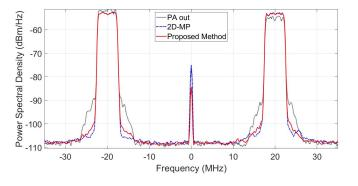
Fig. 6. Linearization performance of the proposed method.
