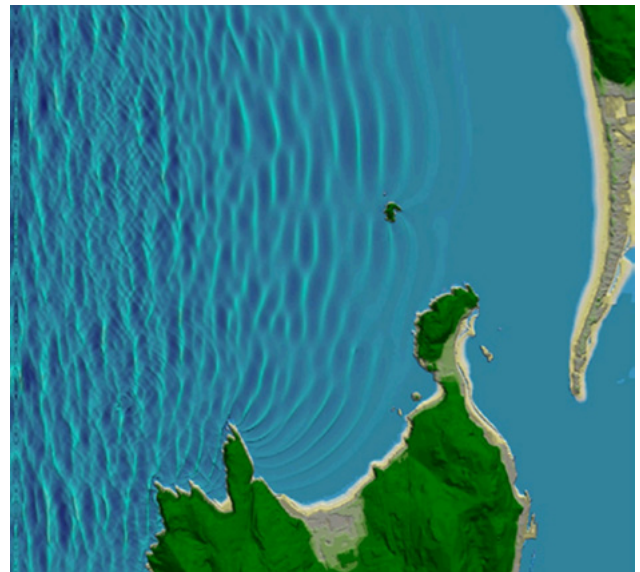
Figure 8.23. Free surface snapshot from the FUNWAVE-TVD applied in Sardinero Beach and Santander Bay (Spain) outer and inner zone (source: University of Cantabria).
