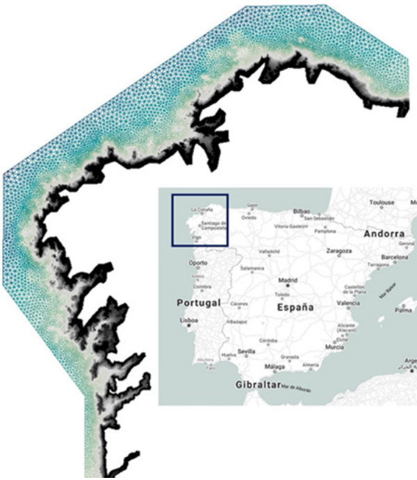
Figure 8.26. Finite Element Method (FEM) based on irregular sized triangles applied to Galicia (Spain) for SWAN model (source: University of Cantabria).
