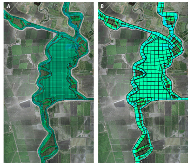
Figure 3.3. Comparison between high-resolution (left) and coarse-resolution (right) from the Bay-Delta model grids by the UnTRIM model in the region of Mildred Island, San Francisco Estuary, U.S., showing the savings in resolution with little loss in accuracy by the application of sub-grid-scale bathymetry parameterization – from MacWilliams et al. (2016).
